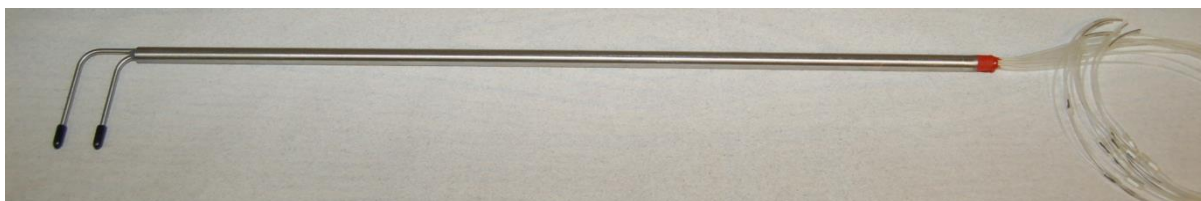
Figure 6. Two-element, 5-hole probe rake.
