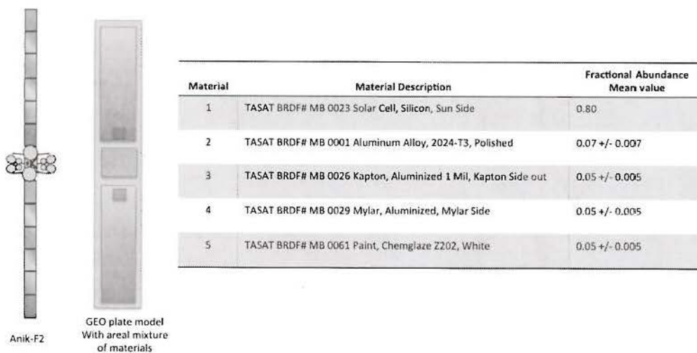
Figure 3 A statistical model of a GEO satellite with the FA of surface materials in the table modeled using a Gaussian distribution
