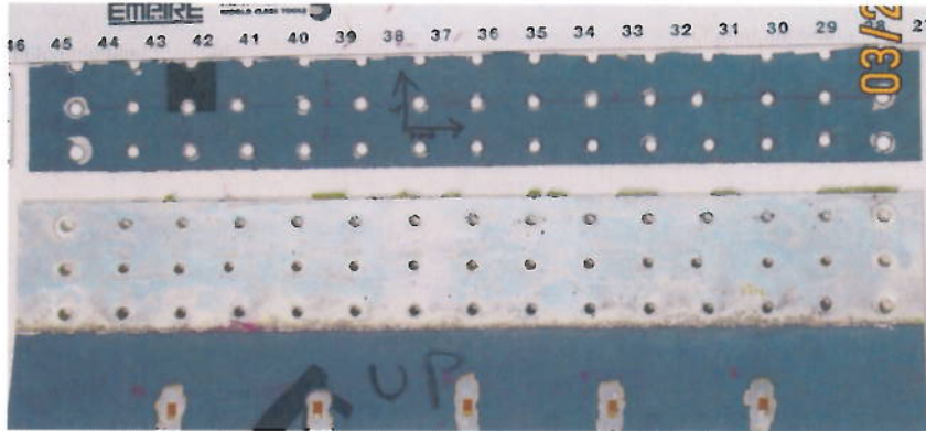
Figure 6: Failure of the test panel at the top most row of the fasteners (nearest the scale; scale in inches). It can be seen that the bottom panel is completely intact.
