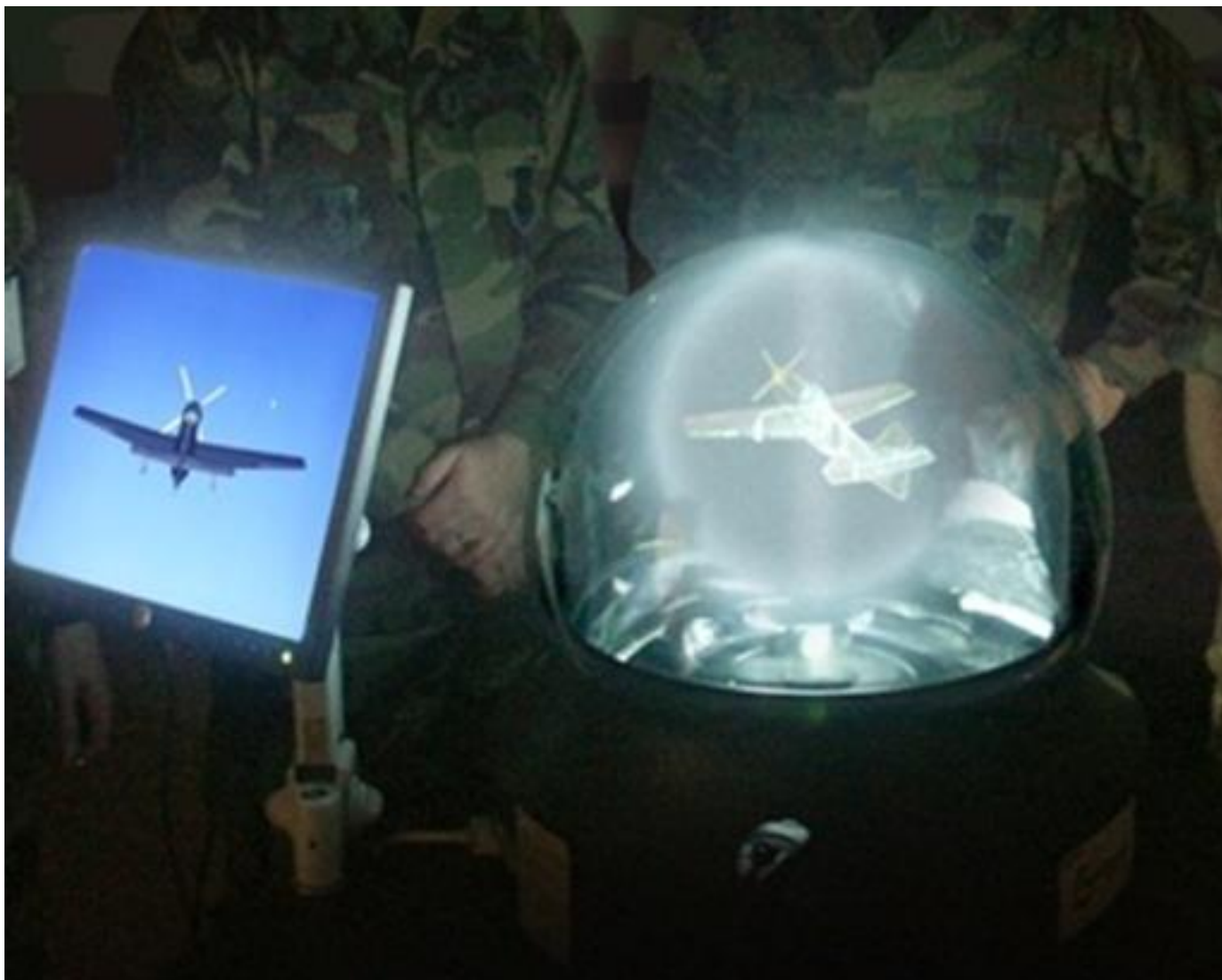
Figure 11. Aircraft Model Displayed in 2D on Flat Panel (left) vs. in 3D on AIS Perspecta (right)
