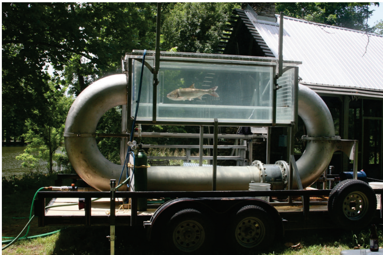
Figure 2. ERDC Mobile Swim Tunnel at Forest Home Chute, a backwater – channel of the Mississippi River near Vicksburg, Mississippi. Inflow is located on the left side, outflow is located on the right side. The collimator grid can be seen at right.
