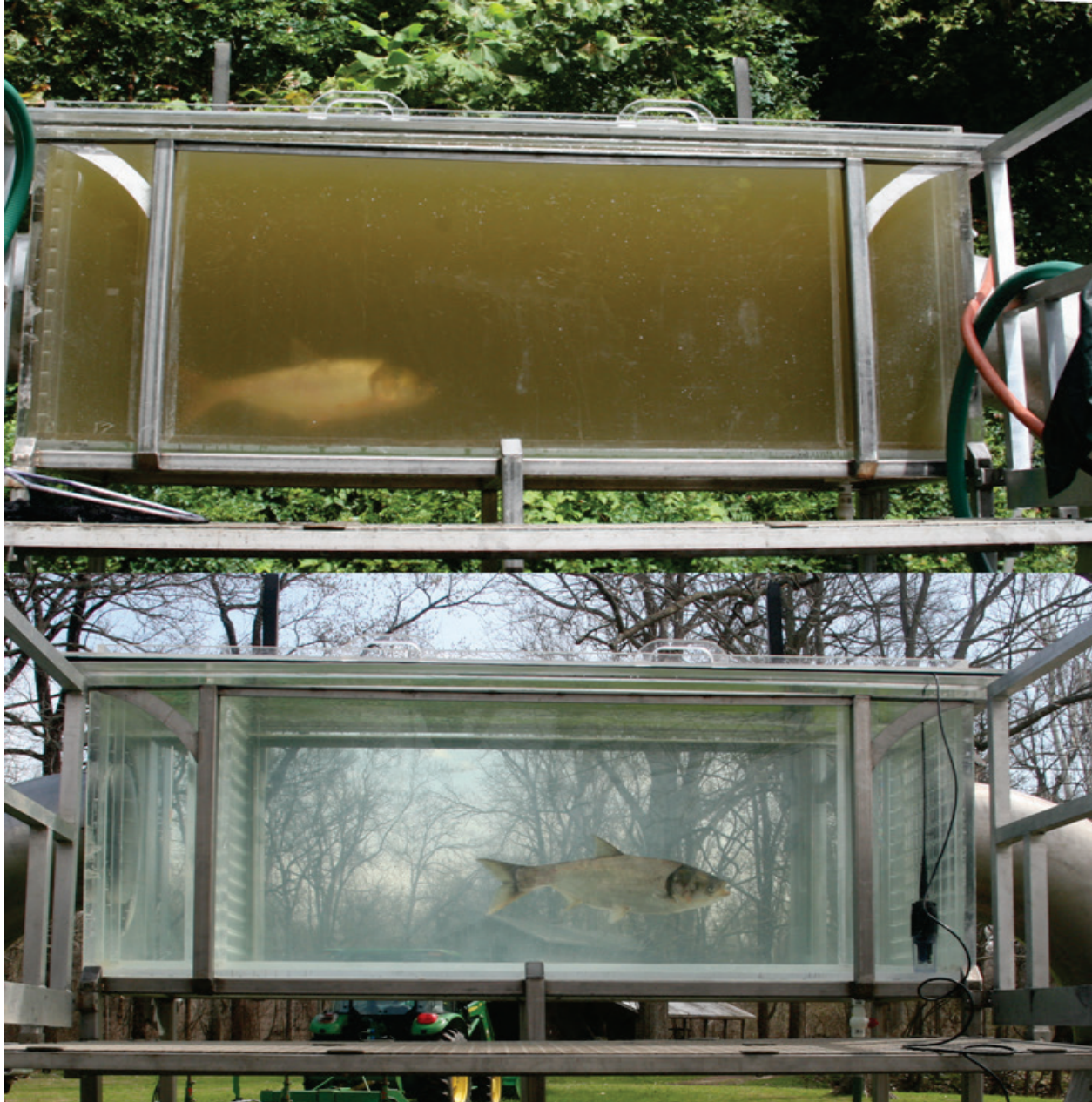
Figure 3. Variation in water clarity. Turbidity was > 40 NTUs during first swim trials (upper) but can be reduced to < 20 NTUs with on-site filtration, and < 2 NTUs with the use of on-site tap water comparable in water quality (conductivity, pH, etc.) to river water (lower).
