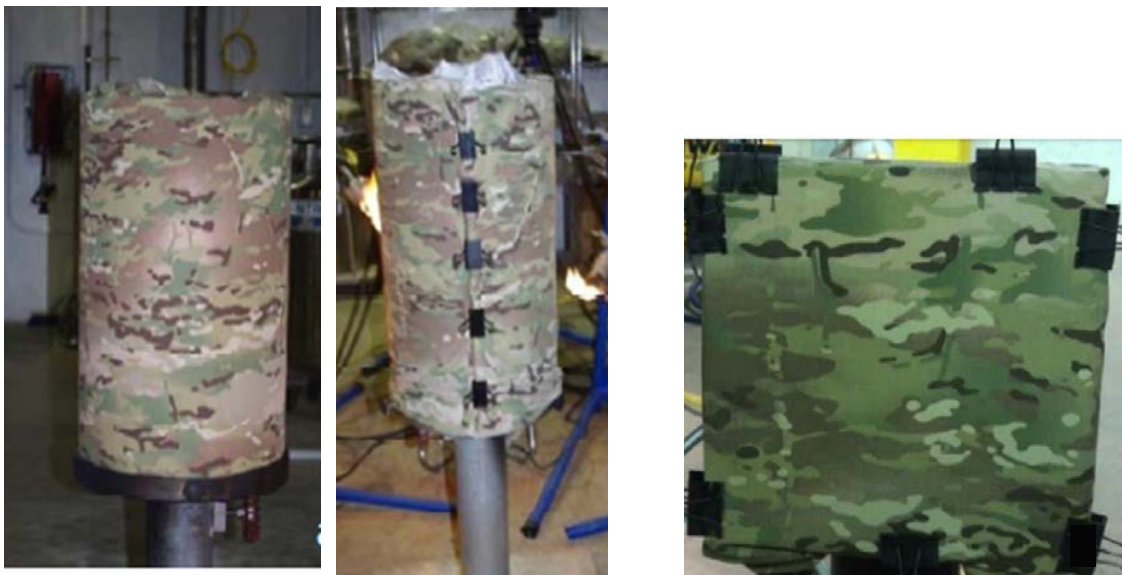
Figure 8. Clamping of fabric specimen: cylindrical and flat plate test forms
