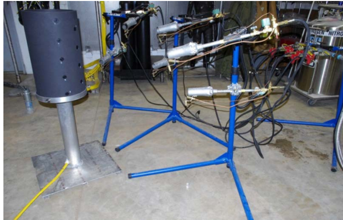
Figure 6. Cylindrical test form with eight burners/four stands
