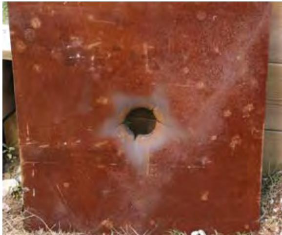
Penetration Hole in 0.5-in. RHA Steel
