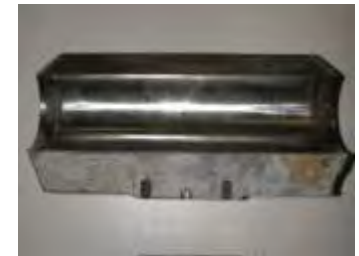
Chamber failed in fatigue
