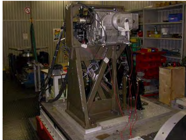
Feed System on Vibration Table November 2004
