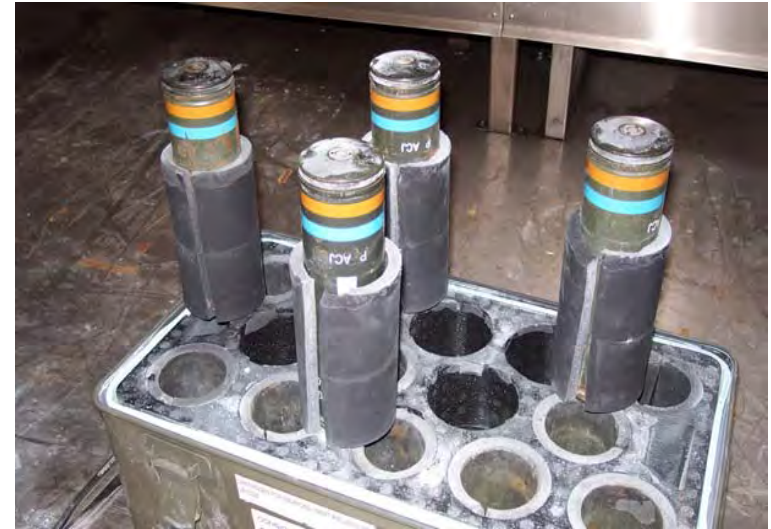
Some Deterioration of Packaging
