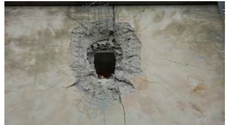
Exit Hole, Test PGM-C02 7" 5K RC 30° obliquity
