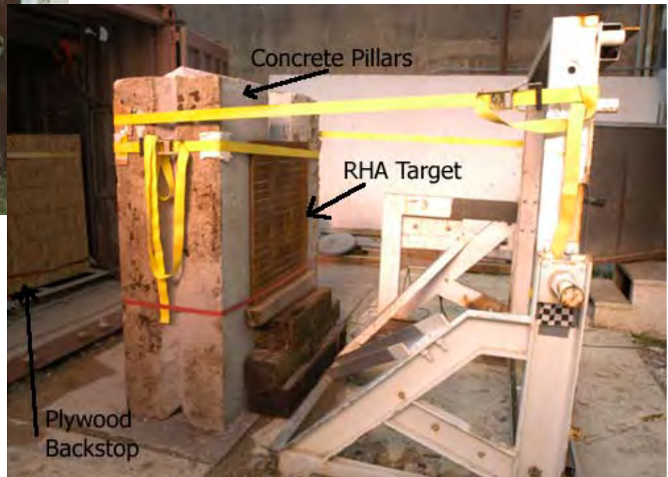
Normal Impact RHA Steel Target Setup
