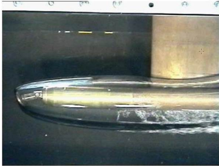
Figure 1.1: Supercavitating vehicle in a water tunnel with a smooth cavity surface.
