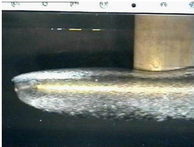
Figure 1.2: Supercavitating vehicle in a water tunnel with a rough and bubbly cavity surface.
