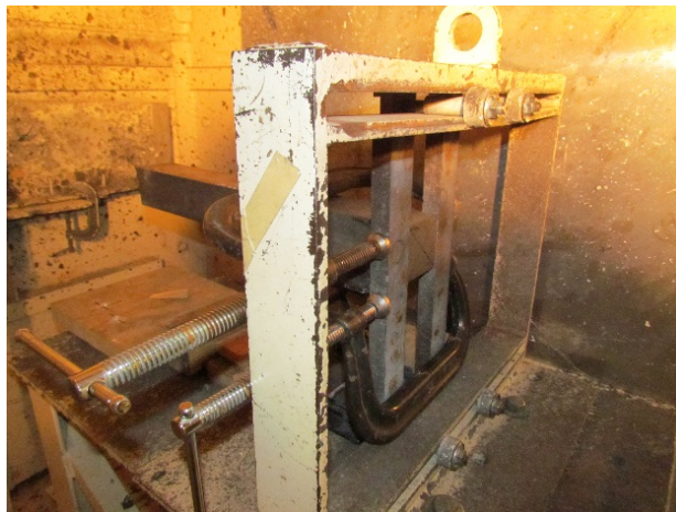
Fig. 5 Experimental target fixture with plate oriented in transverse direction for testing
