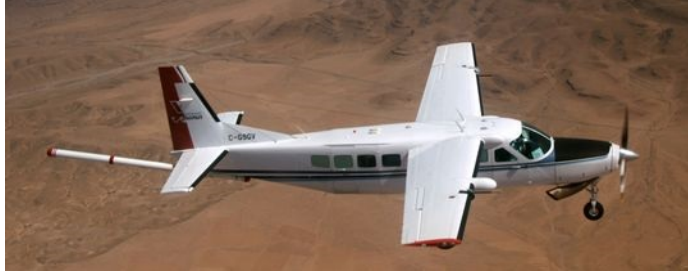
Figure 34. Aircraft Stinger Holding Magnetometer [22]
