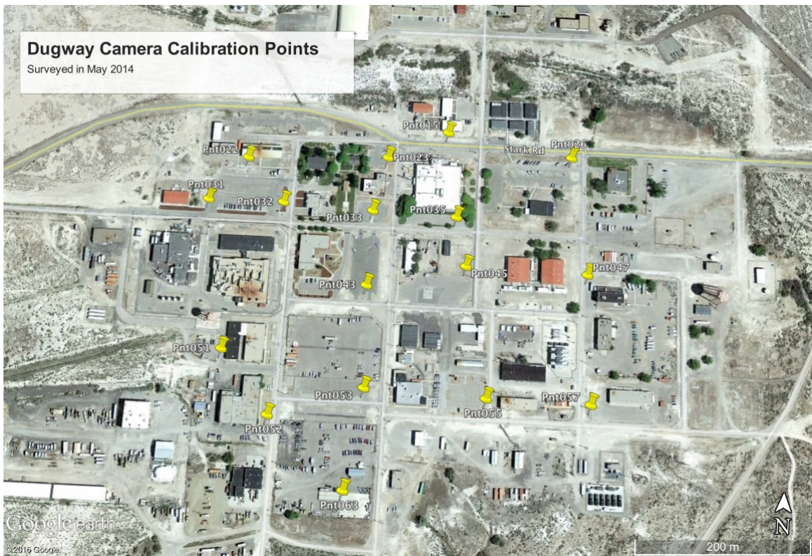
Figure 24: Manually surveyed camera calibration world-points around Dugway Proving Grounds. Image provided by Google.
