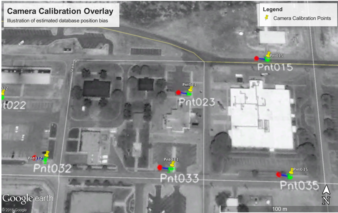
Figure 30: Illustration of landmark database position bias estimate. Push-pins represent the manually surveyed locations of calibration points. Red circles show the projection of these calibration points onto the reference satellite image used to initialize the landmark database, using the provided projection metadata. Green circles show the projection of the calibration points onto the reference image when corrected using the global bias estimate from the camera autocalibration algorithm.
