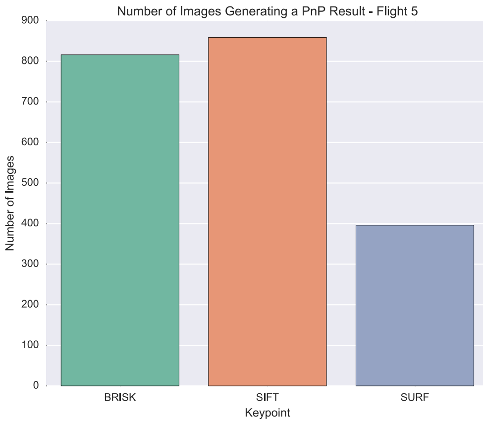
Figure 35: Number of images in Flight Campaign 2, Flight 5 which generated a pose estimate from PnP.
