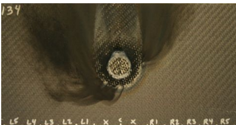
Fig. 27. Large test panels at 85, 284, and 490 W/cm 2 . Backside in inset. Markings are guidelines for cutting into testing strips (later widened strips, allowing only 4 to be cut).
