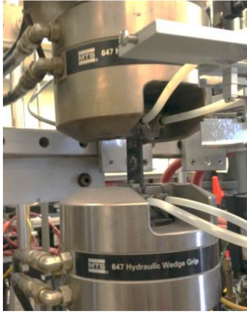
Fig. 25. MTS Testing Machine with sample.
