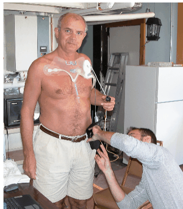
Fig. 2. Example of noninvasive physiological sensors (Nexan Ltd.), which can transmit data wirelessly via an attached PDA. Measures 2-lead electrocardiogram, pulse oximetry, heart rate, respiration rate and temperature.
