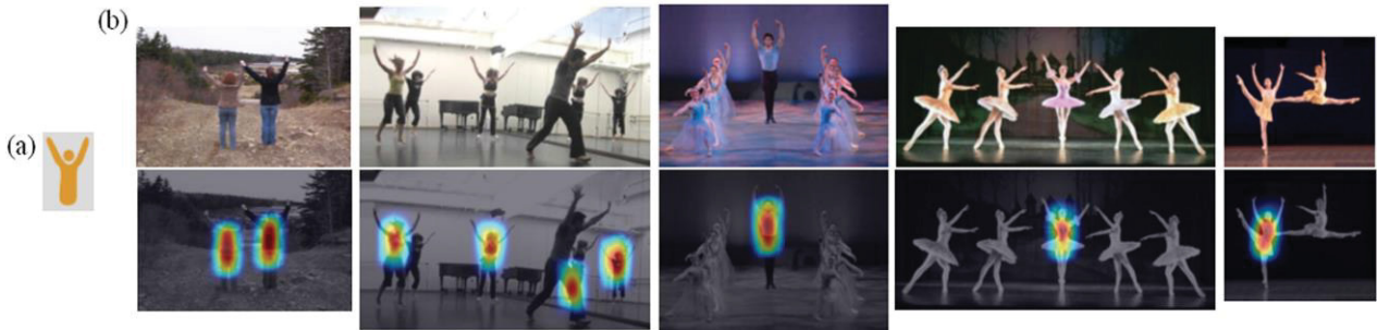
Figure 2-6 Detection of a Person Raising Both Arms (a) A Hand-sketched Template (b) Detected Locations in Other Images (Source: [P-13])
