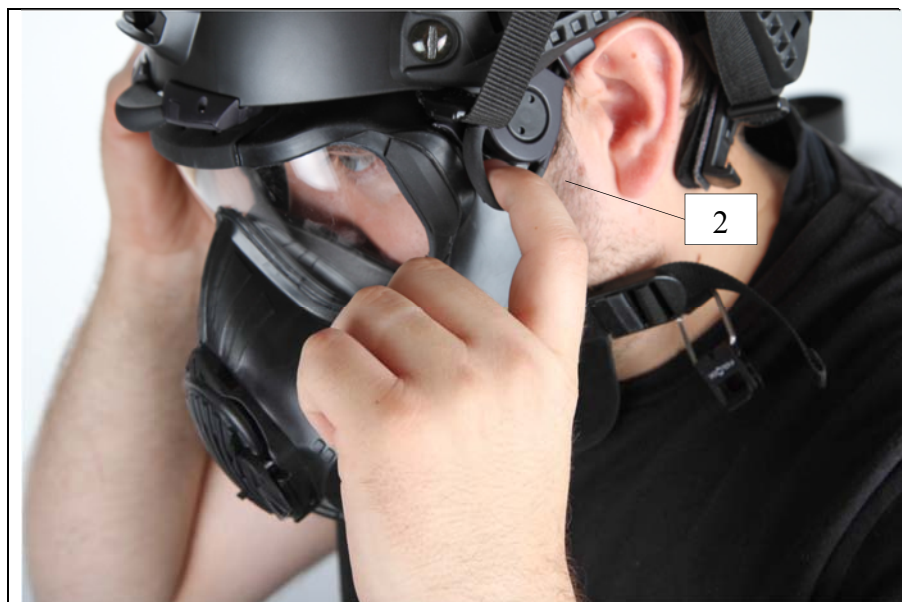
Figure 2. Step 2: Integrated system donning procedures. Next, the volunteer located the molded loops on the temple area fasteners and pulled them forward into position against elastic tension. Magnets within this fastener hardware were used to help guide the fastener to the receiver located on the mask.
