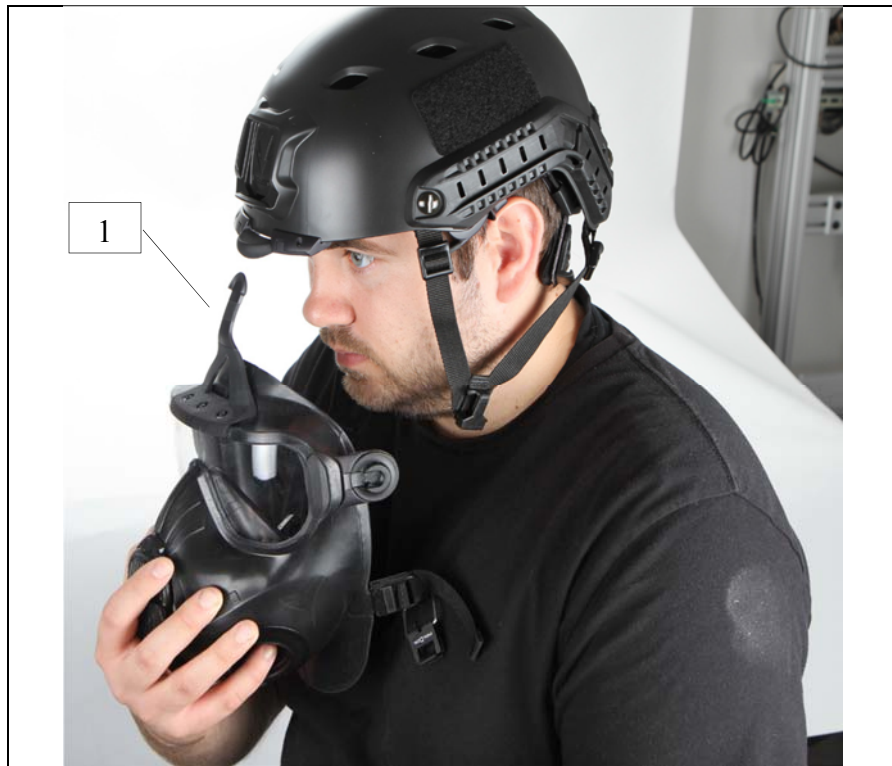
Figure 1. Step 1: Integrated system donning procedures. The volunteer put on the helmet first but left the chin strap detached. A forehead latch tab built into the C50 mask was guided into position in a forehead latch mechanism that was built into the helmet.
