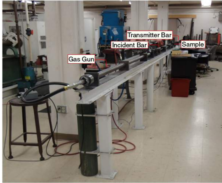
Figure 13. Split Hopkinson Bar test apparatus located at UDRI used for higher temperature and strain rate experiments
