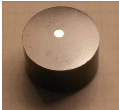
Figure 41. Final product of sample preparation: Sample has been sectioned, mounted, ground, and polished to a 0.05\mu\text{m} surface finish
