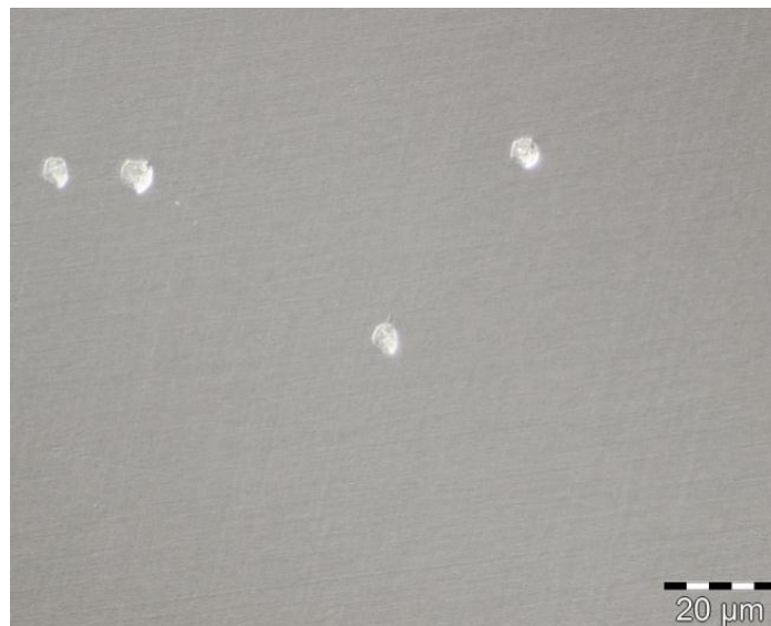
Figure 5-7: Void defects observed on a \text{Hg}_{1-x}\text{Cd}_x\text{Te} imaged by Nomarski x100. Taken from Reference [10].
