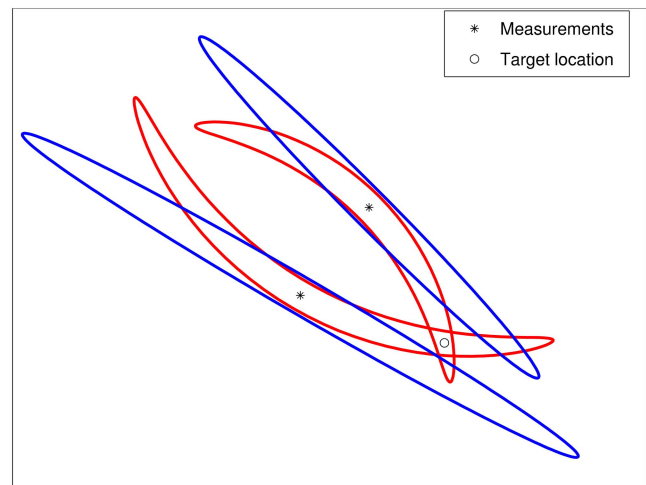
Fig. 3. Gaussian-approximated versus actual (crescent) uncertainty regions. In Gaussian approximation, target-originated measurements will be ignored.
