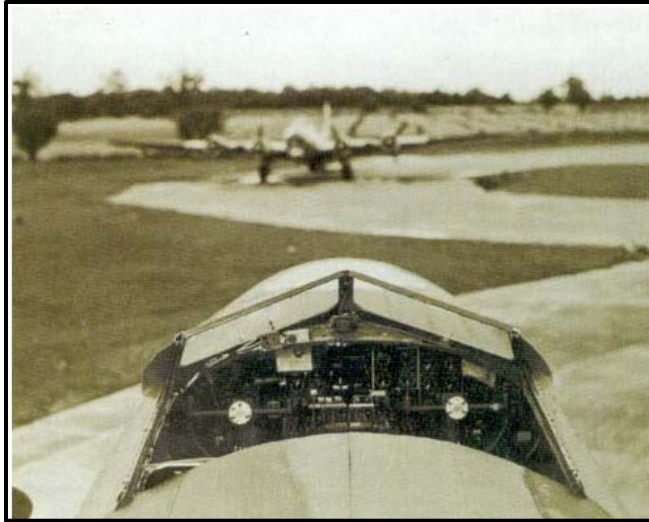
Figure 5. B-17 Drone (BQ-7) Cockpit
