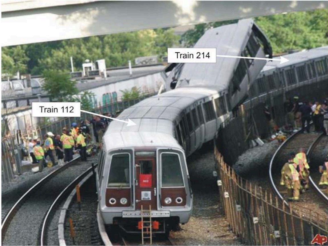
Figure 9. Lead Car of Striking Train (Train 112) has Overridden the Last Car of Struck Train (Train 214), which has Telescoped into the Lead Car of Train 112
