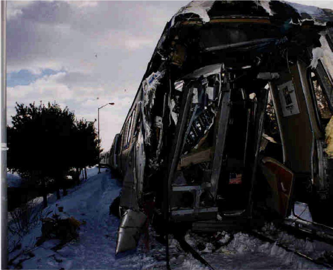
Figure 5. Figure 5. Head end of Train T-111 during Shady Grove Accident, where Operator's Unit was Completely Crushed
