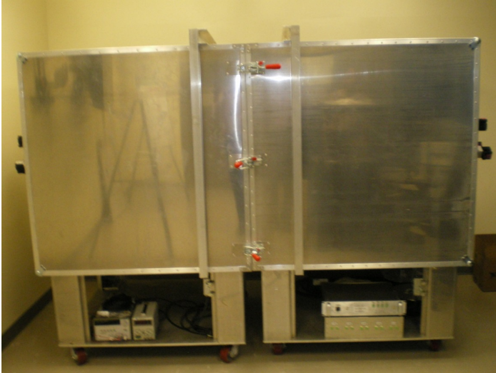
Fig. 3 Aluminum RF section showing clamps available for opening the chamber
