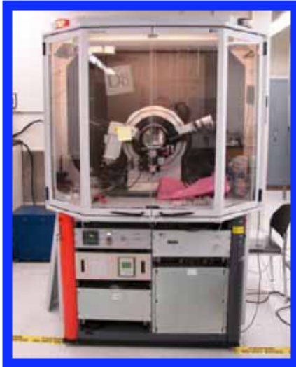
High Temperature X-Ray Diffractometer (up to 1500K)
