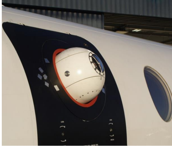
Figure 23: The AAOL turret installed on AAOL-T, left and the instrumented optical bench, right.
