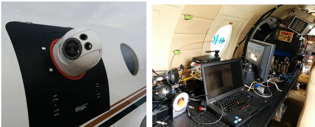
Figure 4. The AAOL turret installed on AAOL-T, left and the instrumented optical bench, right.
