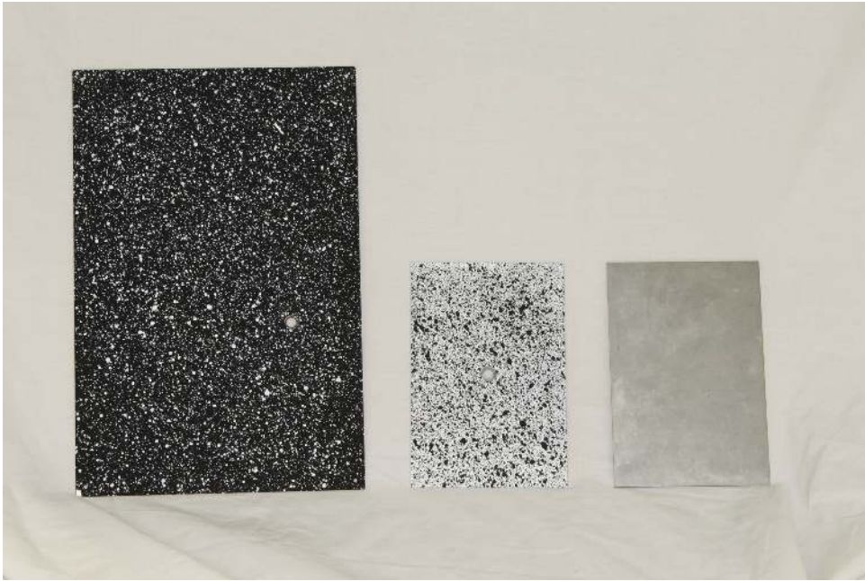
Figure 3.1: One of the large plates sprayed with a base coat of black paint and white speckle. The small plate in the middle has a base coat of white with a black speckle. The small plate on the right is un-painted.
