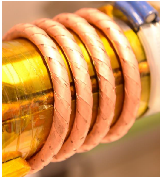
Figure 10. The sample holder including the cable, showing the strong deformation (buckling) of the tapes due to the small bending radius.
