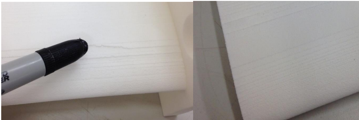
Figure 38. Illustration of a “bad” skin surface finish.
