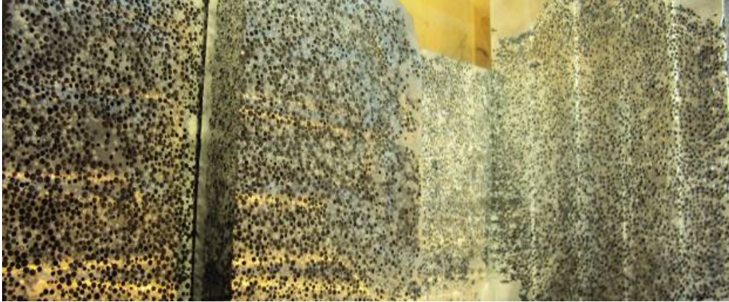
Fig. 26 SiC hollow-sphere-filled AA5083 syntactic metal matrix composite 9- × 13-inch plates were cast at various pressures to establish optimum casting conditions
