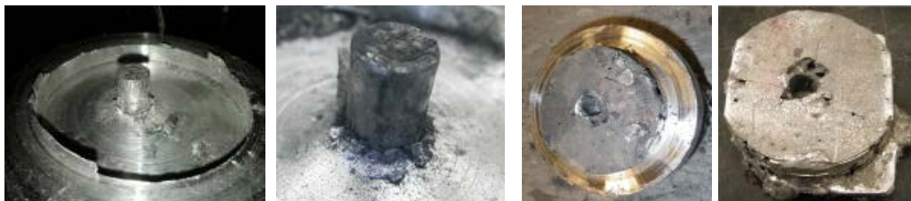
Fig. 63 Images of recovered composite and sabot materials following reverse ballistic experiment at 660 m/s, showing clean penetration of the steel bullet through the Al-SiC composite and the travel of the bullet into the backing sabot material
