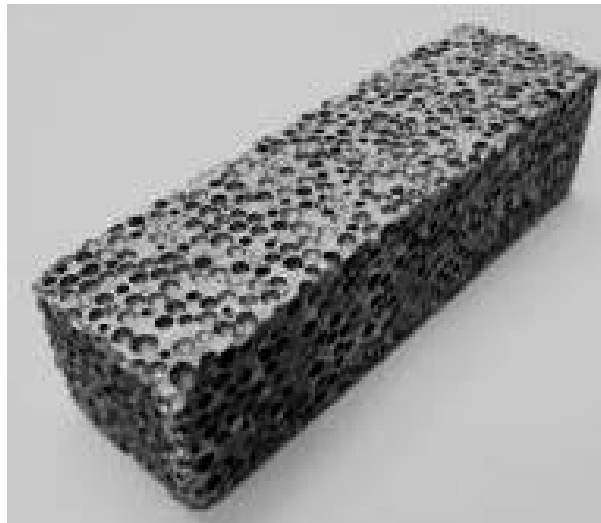
Fig. 7 Buoyancy module featuring SiC and glass hollow spheres in a bimodal distribution
