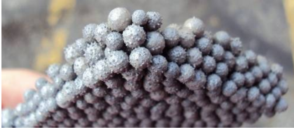
Fig. 21 Densely packed preforms will need to support their own weight during the casting process
