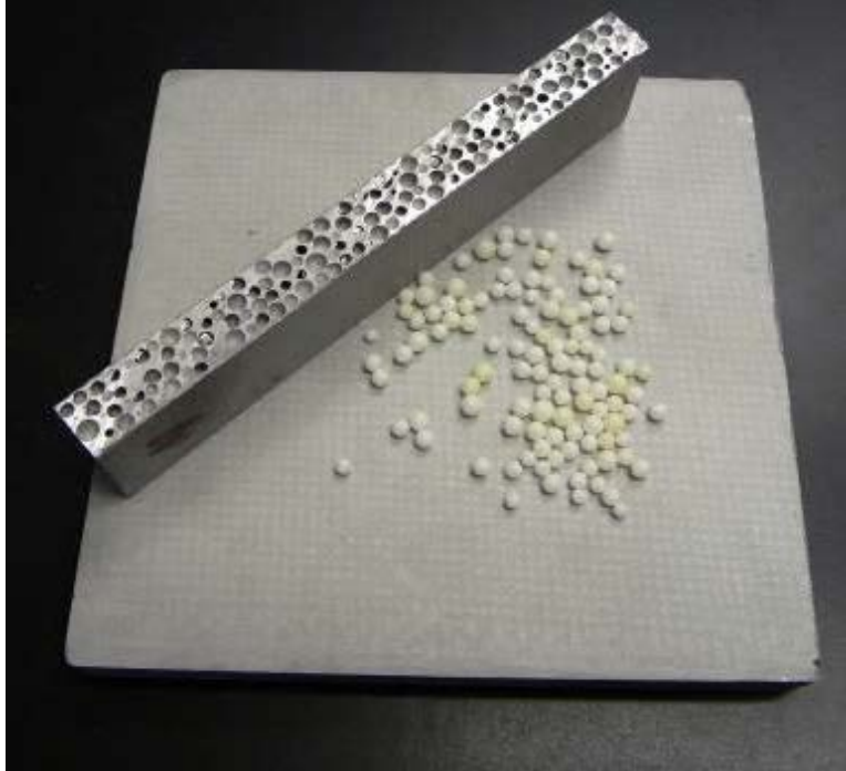
Fig. 71 A356 matrix syntactic foam with 3-mm Al 2 O 3 hollow spheres
