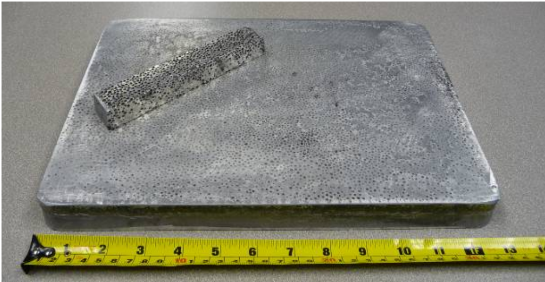
Fig. 50 M350 maraging steel hollow spheres cast into an AA5083 matrix
