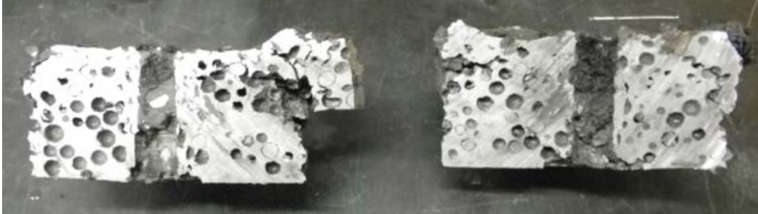
Fig. 64 Cross section of Al-SiC composite penetrated by the 7.62-mm steel bullet at 660 m/s
