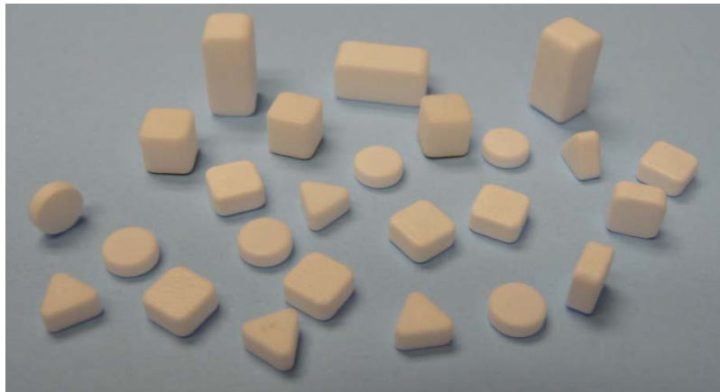
Fig. 4 The variety of hollow shapes that can be produced by DST using their expendable hollow core processing method
