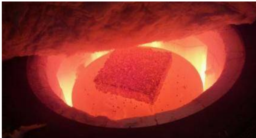
Fig. 22 A preformed block of spheres being preheated prior to casting
