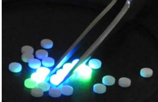
Fig. 12 Short hollow \text{Al}_2\text{O}_3 shells filled with an ionizable gas that has been ignited into a plasma due to presence of an electric field. The maturation of the production process for these shells has allowed their use in syntactic foams.
