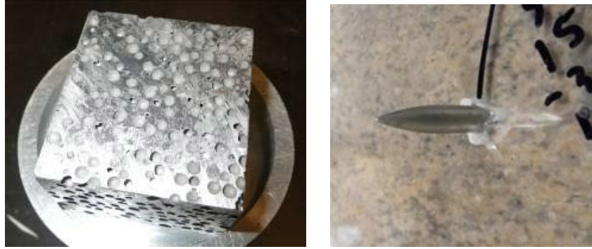
Fig. 62 Composite slab mounted on Al sabot (left) and 7.62-mm steel bullet mounted on PMMA plate (right)
