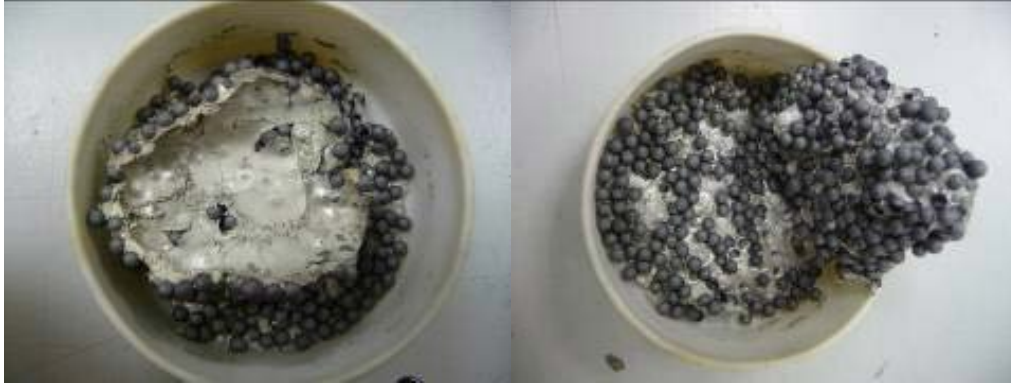
Fig. 17 Layers of aluminum powder and SiC spheres after being fired
