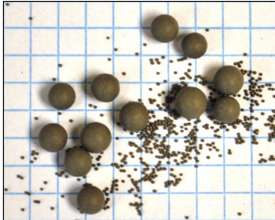
Fig. 9 Hollow SiC spheres were produced with diameters as small as 0.4 mm and larger than 5.9 mm
