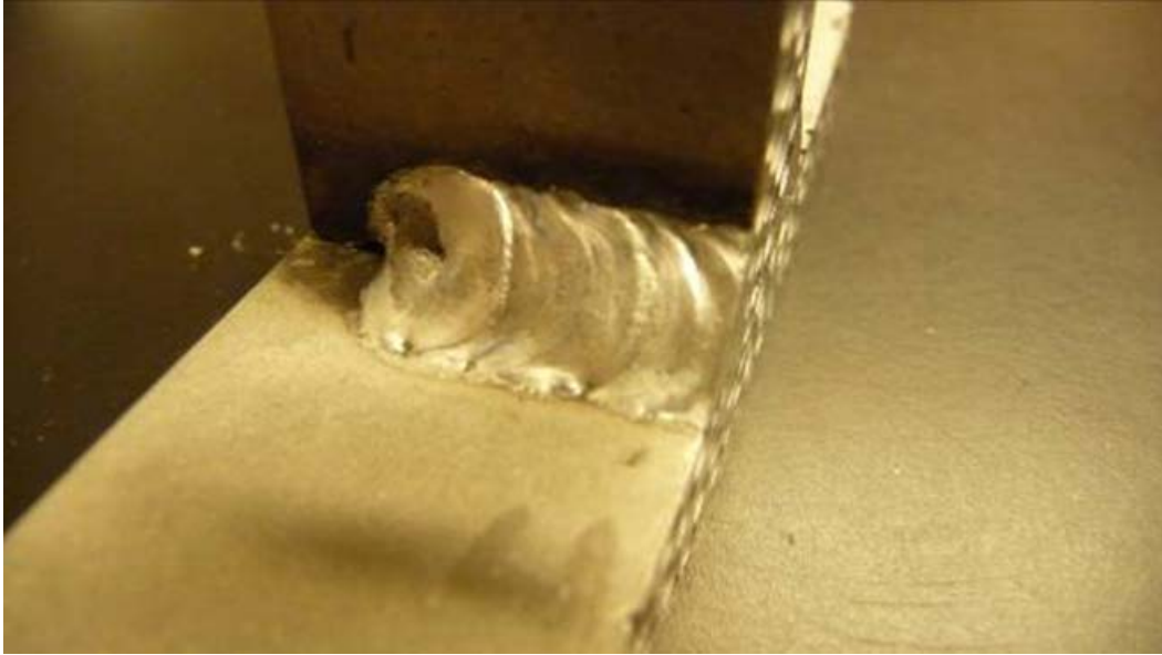
Fig. 74 Weld view: A356/Al 2 O 3 welded panels
