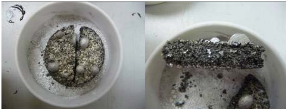
Fig. 18 Sample made from SiC spheres and aluminum powder slurry after being fired
