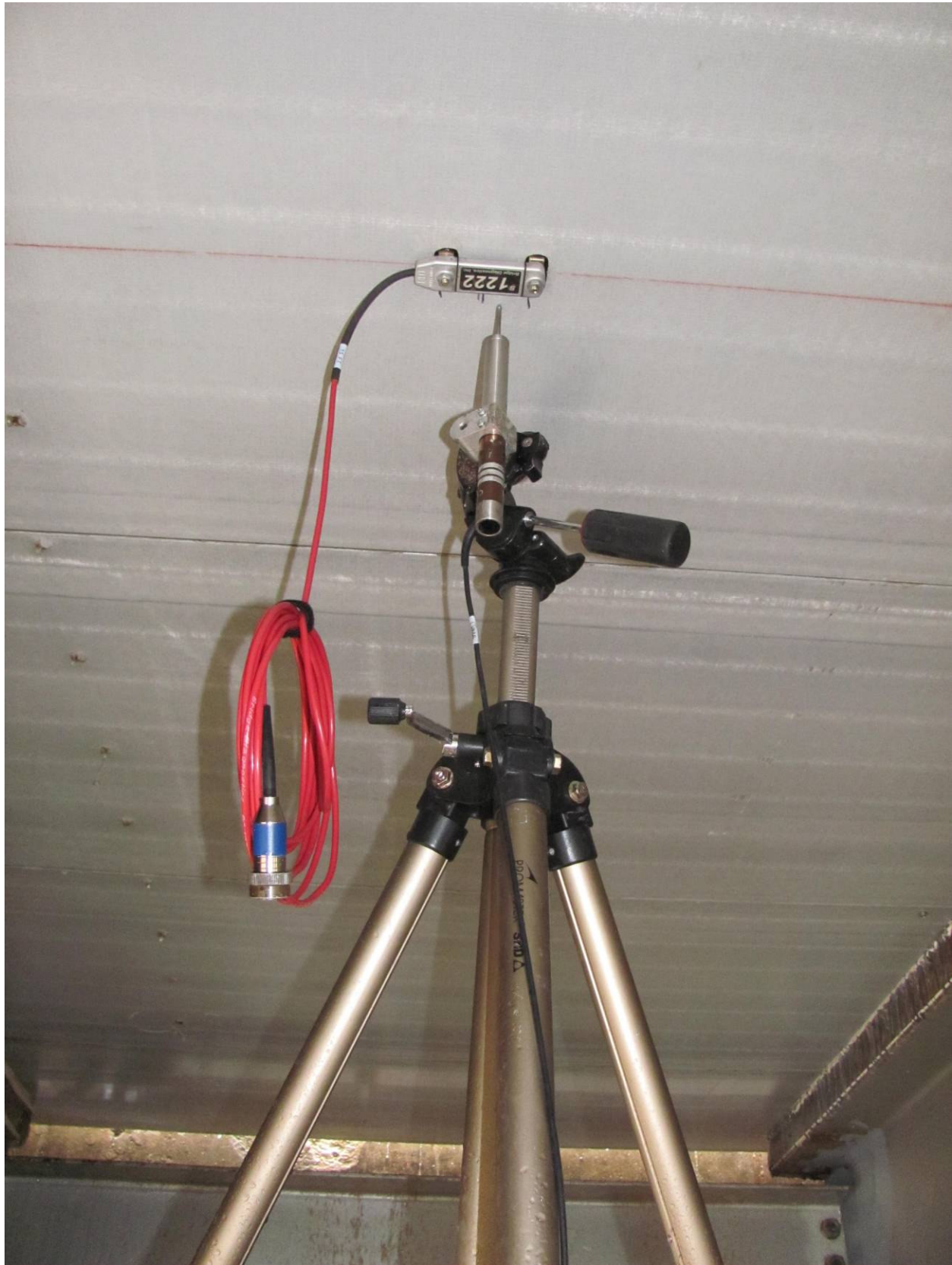
Figure 1.3 Typical strain gage and LVDT at midspan of FRP deck panel.
