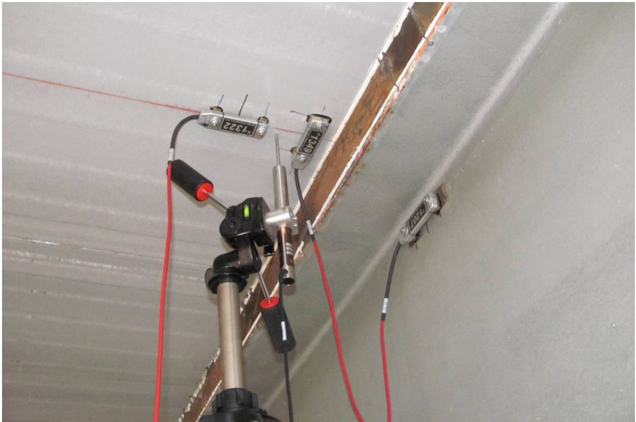
Figure 1.2 Typical strain gages and LVDT at top of beam and edge of FRP deck panel.
