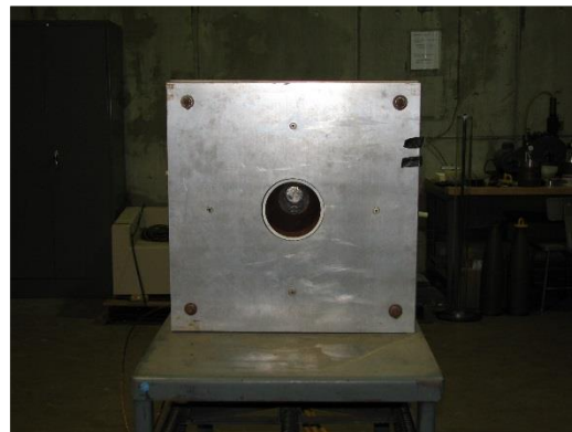
(b) Completed collimator assembly placed within the ARDEC Cf-252 moderator
