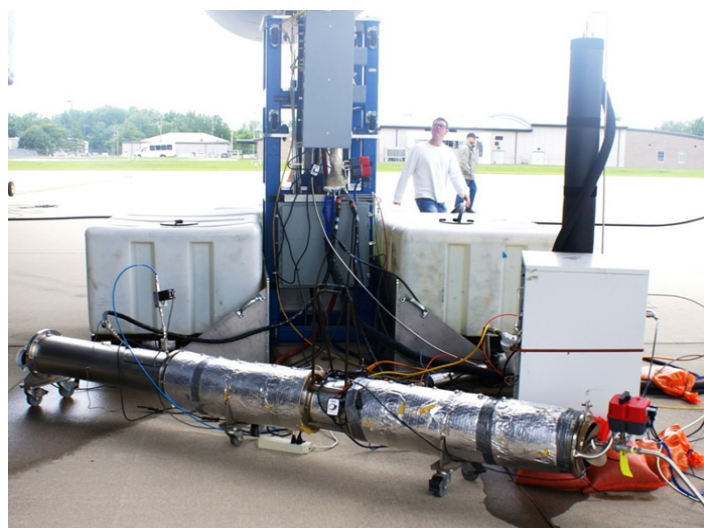
Figure 27. DC and CDP installed near engine during C-17 demonstration
