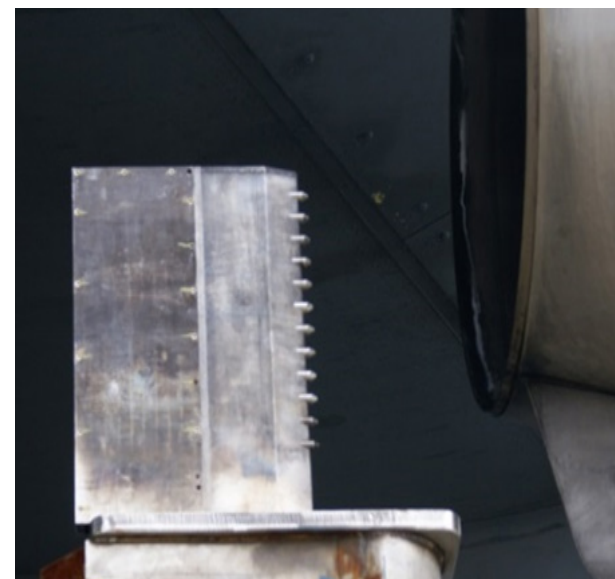
Figure 26. Emissions sampling probes at engine exit, 10m and 20 m, and probe rake for engine exit plane emission sampling
