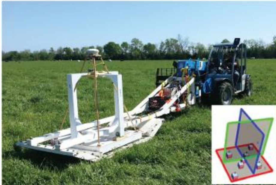
Figure 2-1. Dynamic MetalMapper Deployment at SWPG
