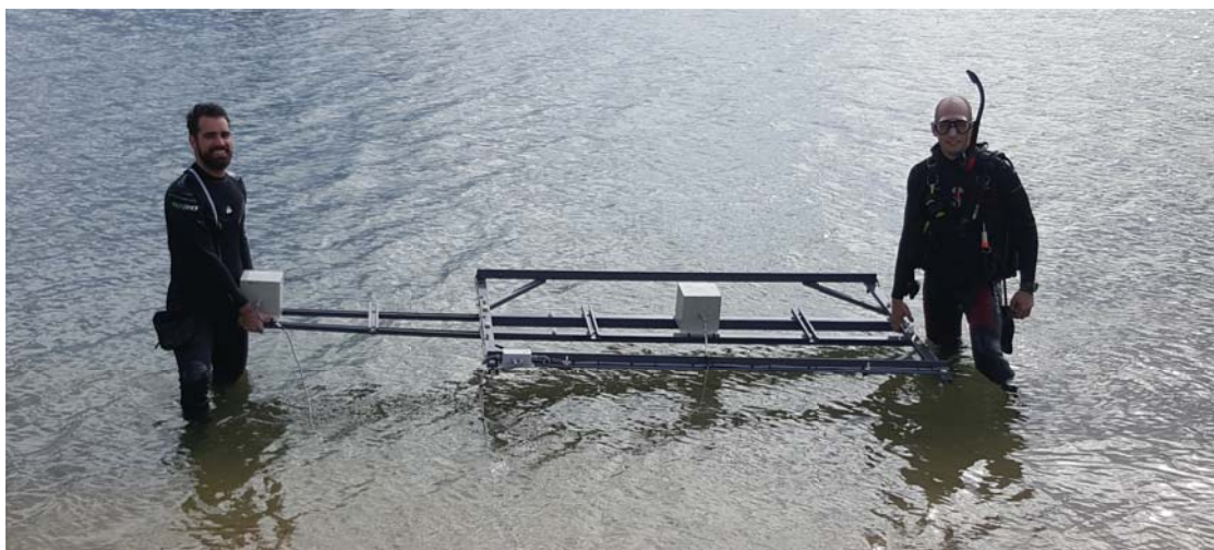
Figure 32: Test frame used for the third measurement campaign. A diver placed the 105 mm projectile at each of the test locations and background measurements were collected before and after each measurement.
