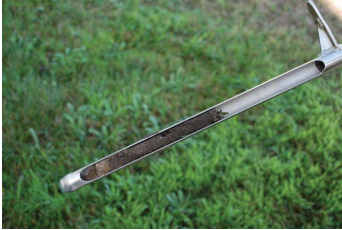
Soil core indicating good moisture penetration and little thatch development
