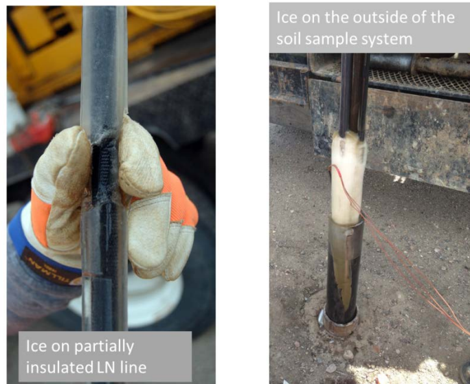
Figure 3-16. Downhole ice locking
