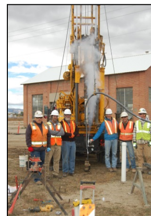
Figure 3-4. Demonstration of cryogenic core collection methods at a former refinery near Casper, WY
