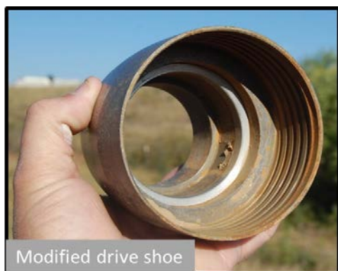
Figure 3-8. Modified drive shoe
