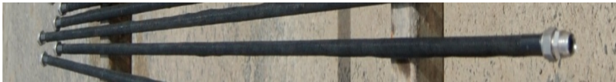
Figure 3-21. Insulated stainless-steel tubes for delivery of liquid nitrogen to core barrels
