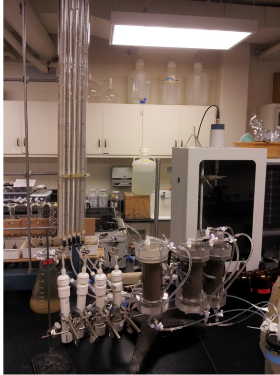
Figure 4-9. Falling head test station
