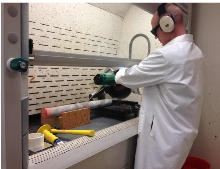
Figure 4-3. Photograph of frozen-core cutting
