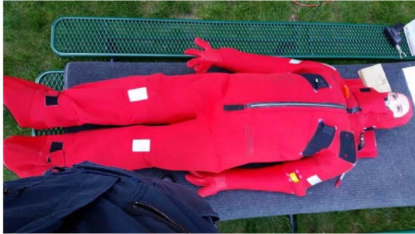
Figure 4. Ballasted mannequin in immersion suit.
