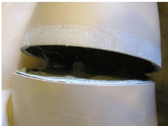
Figure 9. Mannequin leg-joint separation.
