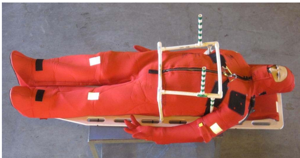
Figure 11. Mannequin in suit with measuring posts.
