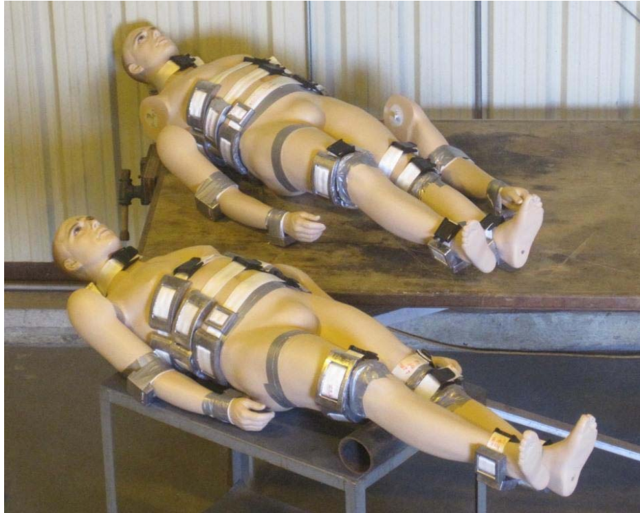
Figure 8. Weighted mannequins before taping at JMTF.
