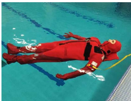
Figure 5. Weighted mannequin/immersion suit flotation trial.
