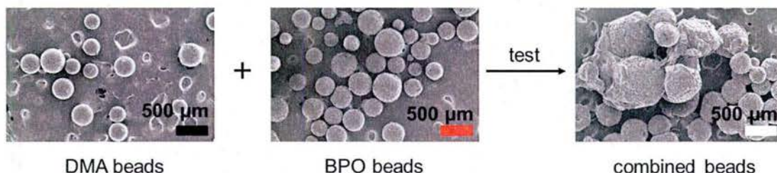
Figure 33. SEM images of individual beads before polymerization test and combined beads after polymerization test.
