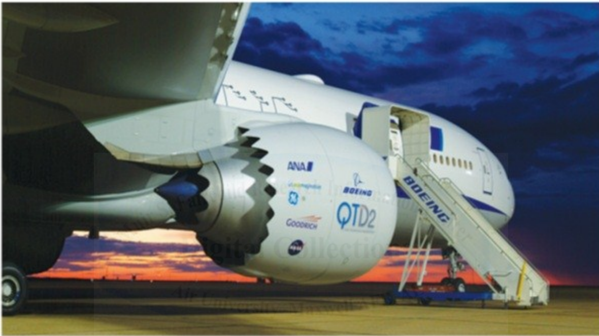
Figure 6: Azimuthally varying chevrons used in QTD2 program (NASA) 30
