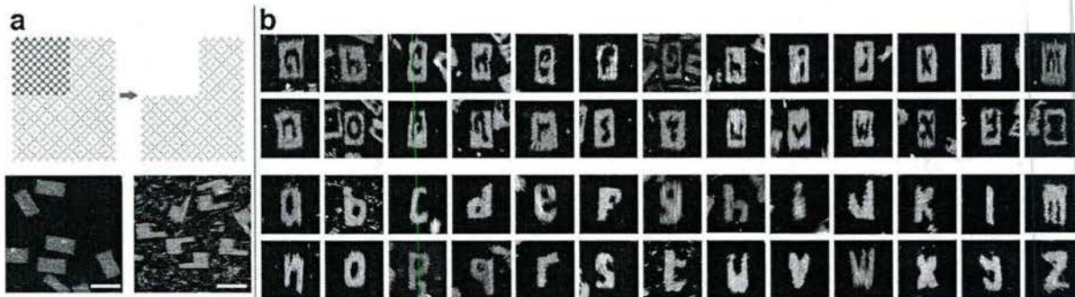
Figure 2. Alphabet sets reconfigured from a rectangular SST canvas. a) Interaction graphs (top) and AFM images (bottom) of the 24 H × 29 T canvas used in this study (left) and its reconfiguration into a rectangle with a missing corner (right). Scale bars: 100 nm. b) AFM images of letters of the alphabet carved in intaglio (top) and relief (bottom). Each image is 150 \times 150 \text{ nm}^2 in size. See Figures S4 and S5 in the Supporting Information for the results of agarose gel electrophoresis.
