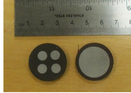
Figure 1. Image of front side (left) and back side (right) electrodes that were sputtered onto each disk.
