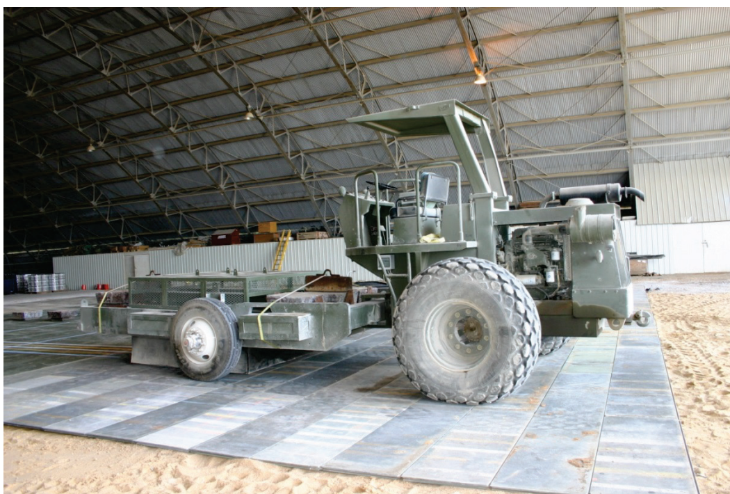
Figure 3.18. F-15E test load cart.
