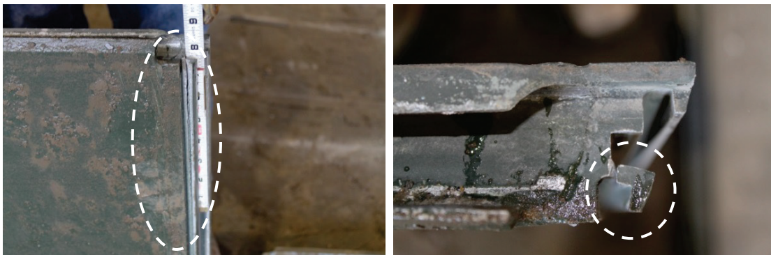
Figure 4.13. Partial breakage of lower overlap rail in G33.
