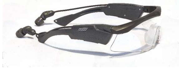
Fig. 1 IEEP device under test: shown with clear ballistic lens and Comply foam earphone tips.
