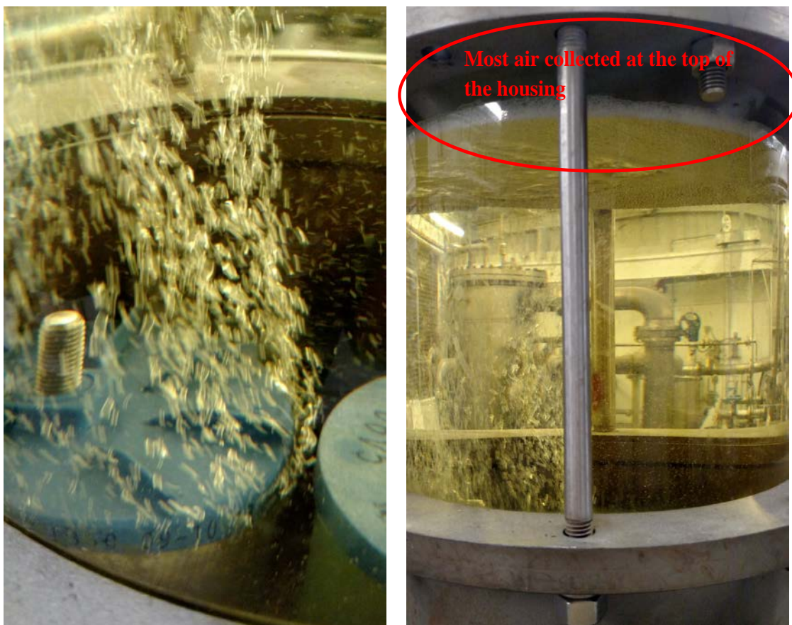
Figure 7. Upstream Air Injection Test Setup – Air Escaping Filter (left) and Air Collecting in Test Housing (Right)
