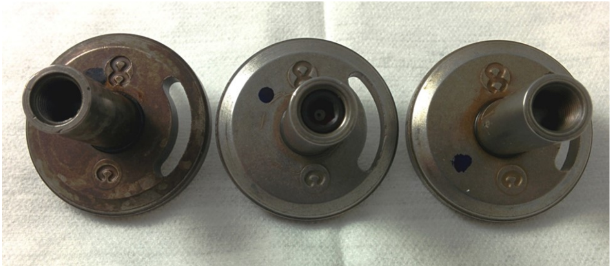
Figure 45. Transfer Pump Endplate Deposition: DSH8 SN:17102938 Endplate Left, ATJ Engine Test Endplate Middle, and DSH8 SN:17102937 Endplate Right
