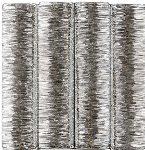
Figure 40. Pump SN:17102938 Transfer Pump Blade Edges with 500-Hours Testing with 20/80 DSH8/JP-8 Fuel with 9-ppm CI/LI
