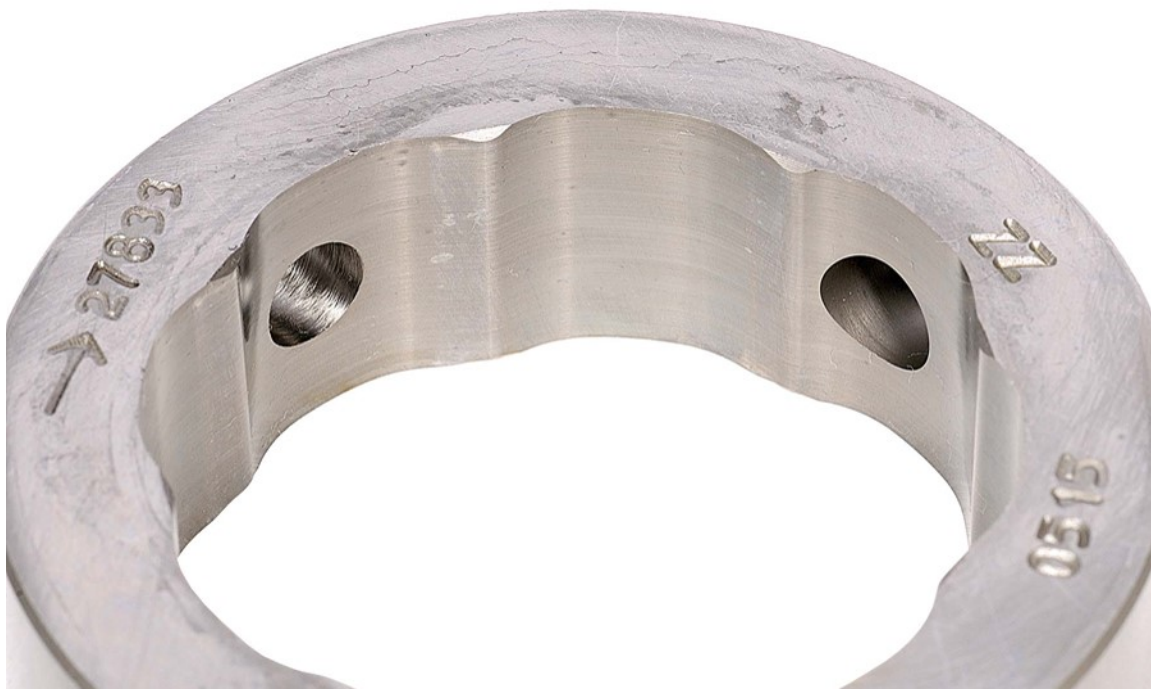
Figure 33. Pump SN:17102938 Cam Ring before Testing with 20/80 DSH8/JP-8 Fuel with 9-ppm CI/LI
