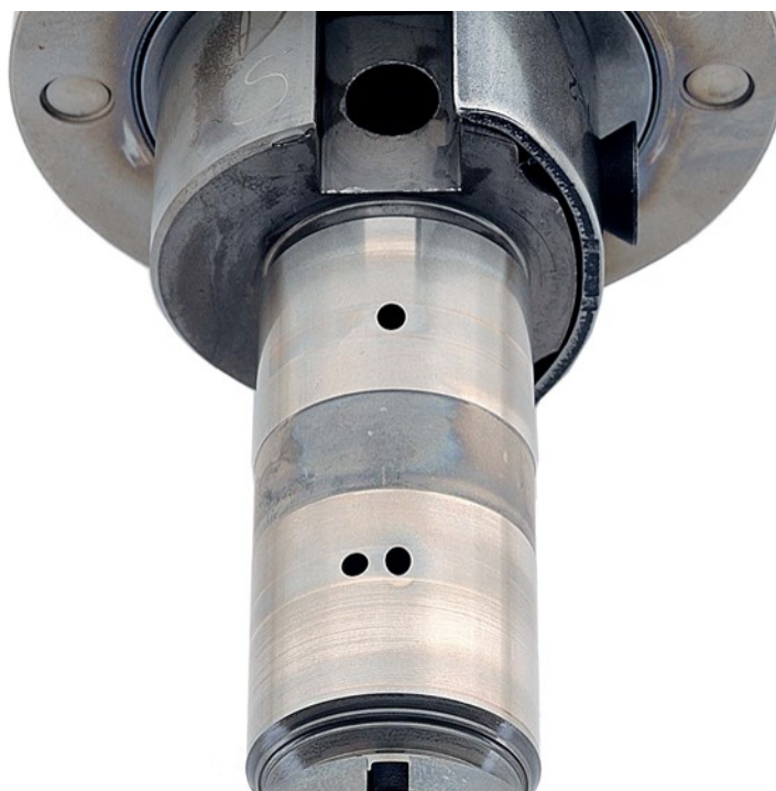
Figure 10. Pump SN:17102937 Distributor Rotor with 500-Hours Testing with 20/80 DSH8/JP-8 Fuel with 9-ppm CI/LI
