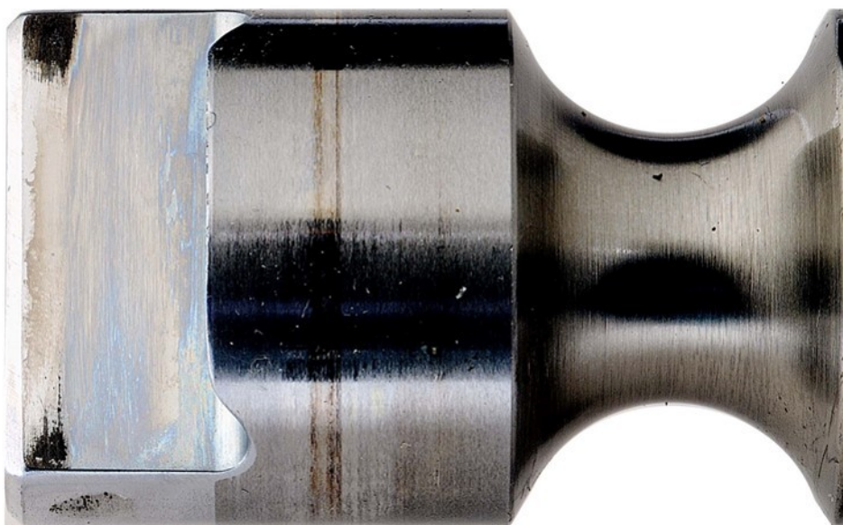
Figure 44. Pump SN:17102938 Driveshaft Drive Tang with 500-Hours Testing with 20/80 DSH8/JP-8 Fuel with 9-ppm CI/LI
