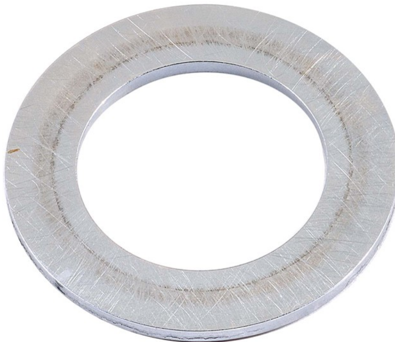
Figure 36. Pump SN:17102938 Thrust Washer with 500-Hours Testing with 20/80 DSH8/JP-8 Fuel with 9-ppm CI/LI
