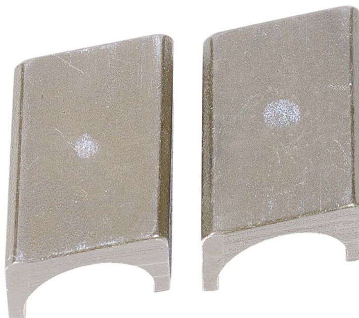
Figure 13. Pump SN:17102937 Roller Shoe before Testing with 20/80 DSH8/JP-8 Fuel with 9-ppm CI/LI
