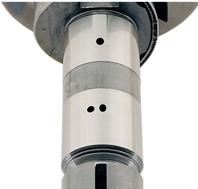
Figure 9. Pump SN:17102937 Distributor Rotor before Testing with 20/80 DSH8/JP-8 Fuel with 9-ppm CI/LI
