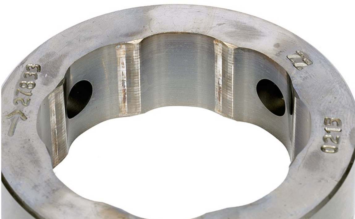
Figure 16. Pump SN:17102937 Cam Ring with 500-Hours Testing with 20/80 DSH8/JP-8 Fuel with 9-ppm CI/LI
