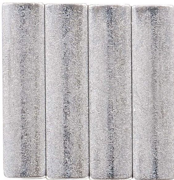
Figure 39. Pump SN:17102938 Transfer Pump Blade Edges before Testing with 20/80 DSH8/JP-8 Fuel with 9-ppm CI/LI
