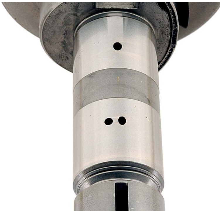
Figure 27. Pump SN:17102938 Distributor Rotor before Testing with 20/80 DSH8/JP-8 Fuel with 9-ppm CI/LI
