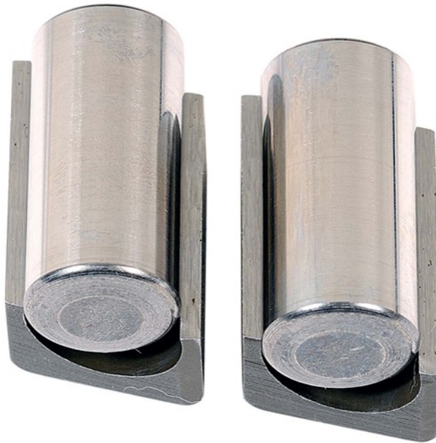
Figure 29. Pump SN:17102938 Rollers and Shoe before Testing with 20/80 DSH8/JP-8 Fuel with 9-ppm CI/LI
