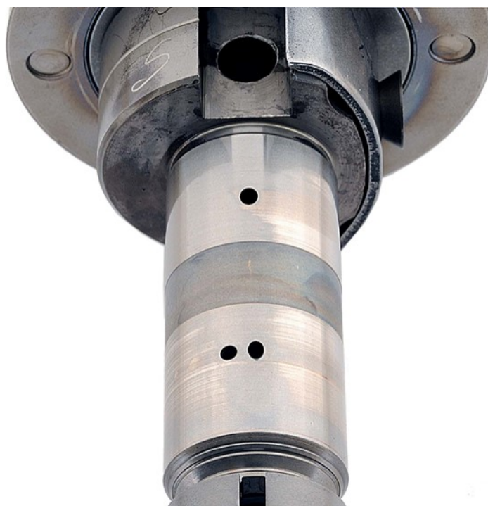
Figure 28. Pump SN:17102938 Distributor Rotor with 500-Hours Testing with 20/80 DSH8/JP-8 Fuel with 9-ppm CI/LI
