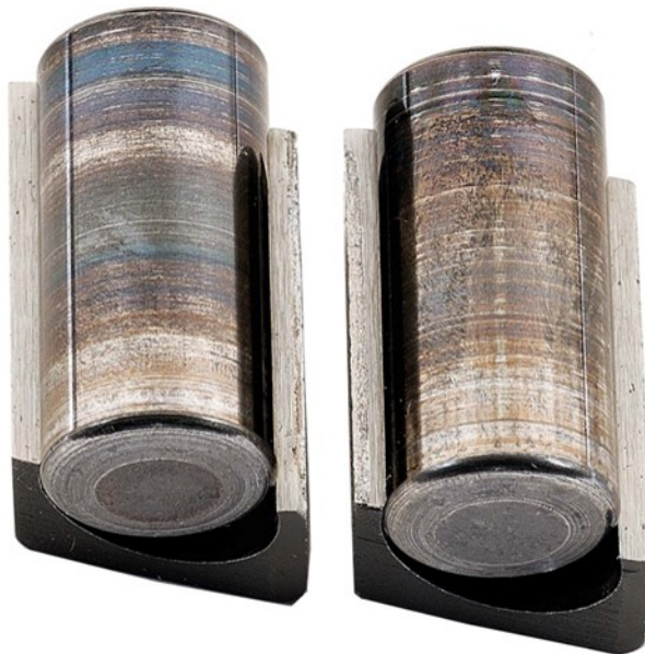
Figure 30 Pump SN:17102938 Rollers and Shoe with 500-Hours Testing with 20/80 DSH8/JP-8 Fuel with 9-ppm CI/LI
