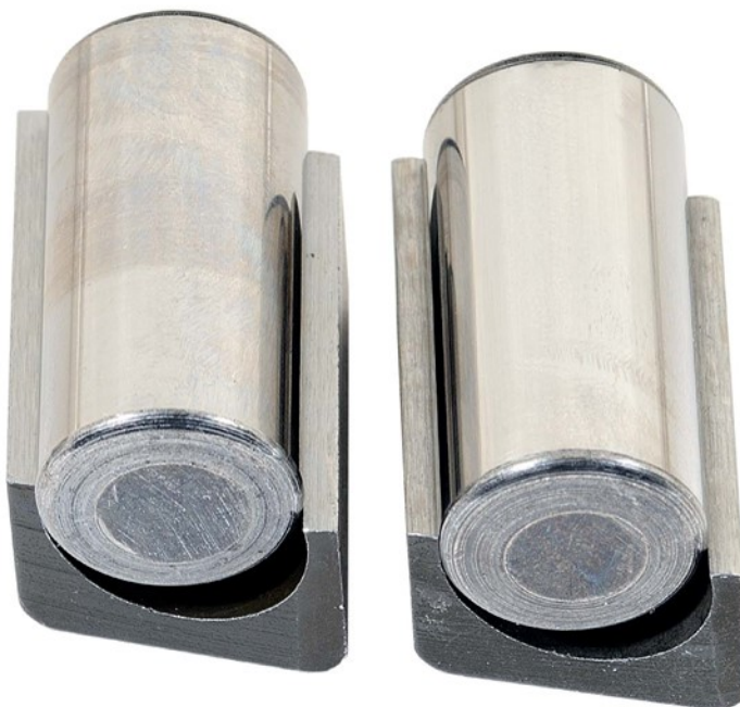
Figure 11. Pump SN:17102937 Rollers and Shoe before Testing with 20/80 DSH8/JP-8 Fuel with 9-ppm CI/LI
