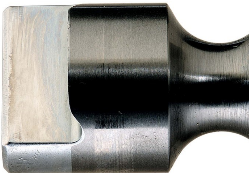
Figure 43. Pump SN:17102938 Driveshaft Drive Tang before Testing with 20/80 DSH8/JP-8 Fuel with 9-ppm CI/LI
