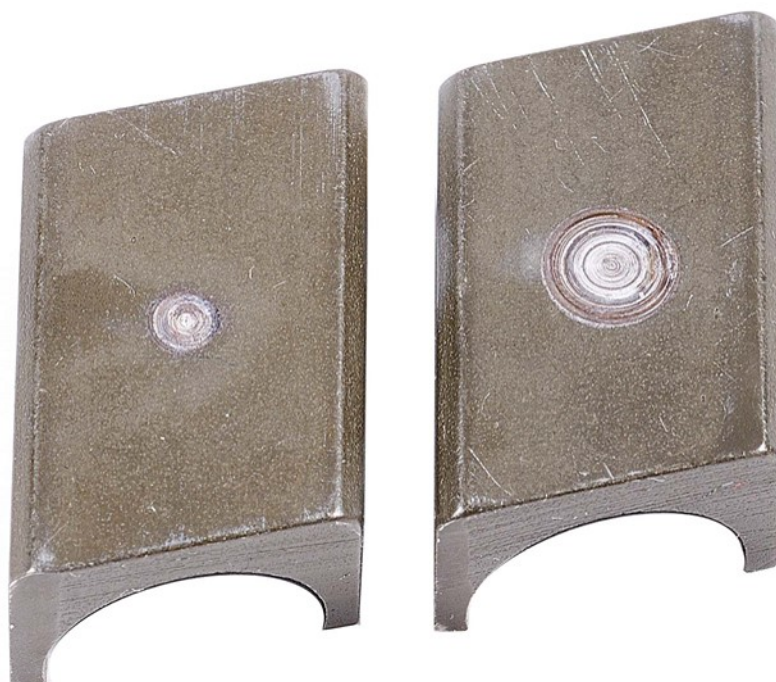
Figure 14. Pump SN:17102937 Roller Shoe with 500-Hours Testing with 20/80 DSH8/JP-8 Fuel with 9-ppm CI/LI
