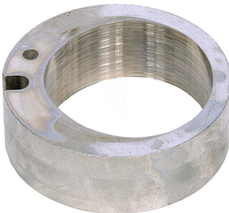
Figure 20. Pump SN:17102937 Transfer Pump Liner with 500-Hours Testing with 20/80 DSH8/JP-8 Fuel with 9-ppm CI/LI
