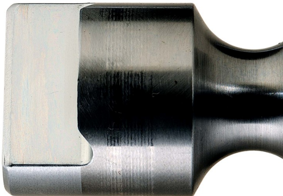
Figure 25. Pump SN:17102937 Driveshaft Drive Tang Sides before Testing with 20/80 DSH8/JP-8 Fuel with 9-ppm CI/LI
