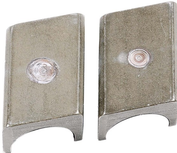
Figure 32. Pump SN:17102938 Roller Shoe with 500-Hours Testing with 20/80 DSH8/JP-8 Fuel with 9-ppm CI/LI
