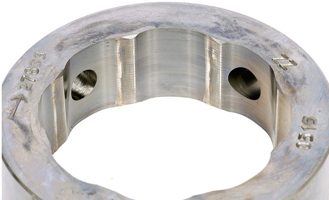
Figure 34. Pump SN:17102938 Cam Ring with 500-Hours Testing with 20/80 DSH8/JP-8 Fuel with 9-ppm CI/LI
