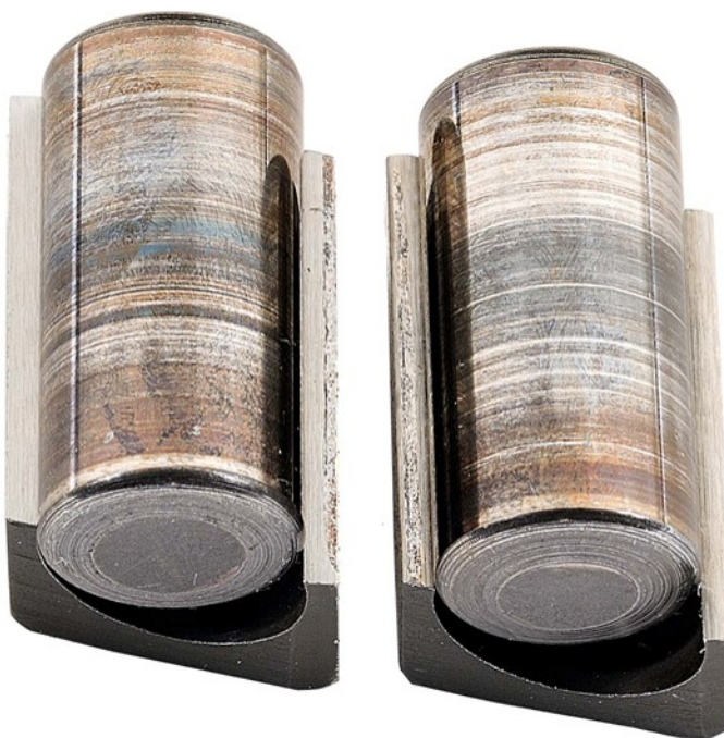
Figure 12. Pump SN:17102937 Rollers and Shoe with 500-Hours Testing with 20/80 DSH8/JP-8 Fuel with 9-ppm CI/LI
