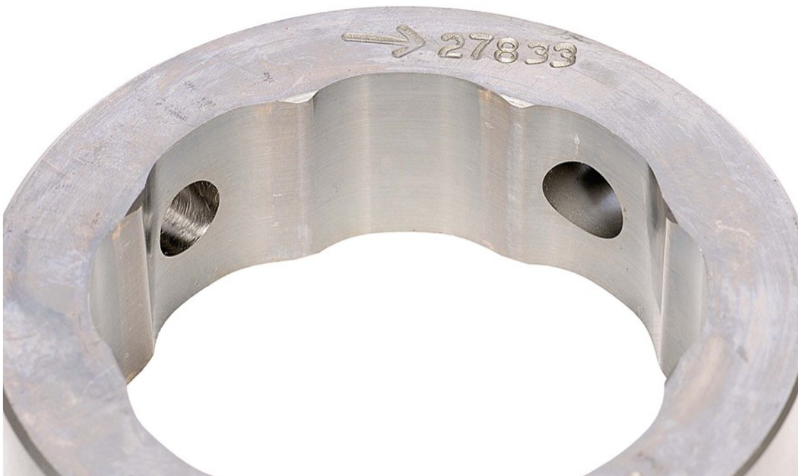
Figure 15. Pump SN:17102937 Cam Ring before Testing with 20/80 DSH8/JP-8 Fuel with 9-ppm CI/LI
