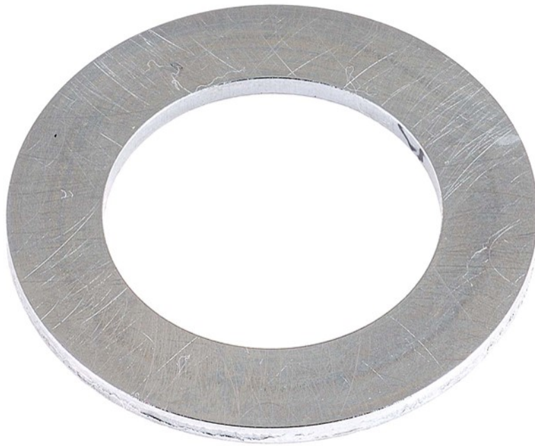
Figure 35. Pump SN:17102938 Thrust Washer before Testing with 20/80 DSH8/JP-8 Fuel with 9-ppm CI/LI
