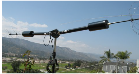
Figure 1: Compact HF-NVIS antenna for vehicle and ground forces (Reproduced by permission of Military Hi-Q [9]).
