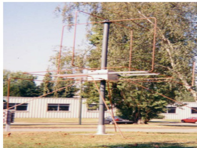
Figure 2: Compact HF direction-finding antenna (Reproduced by permission of the Institution of Engineering & Technology [11]).
