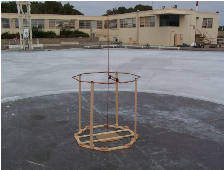
Figure 50: Reference antenna in the SSC Pacific Antenna Pattern Range.
