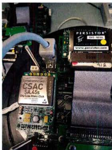
Figure 2. CSAC-SHRU electronic board. A Microsemi Chip Scale Atomic Clock (CSAC) and a PERSISTOR miniature computer are used on the SHRU system.
