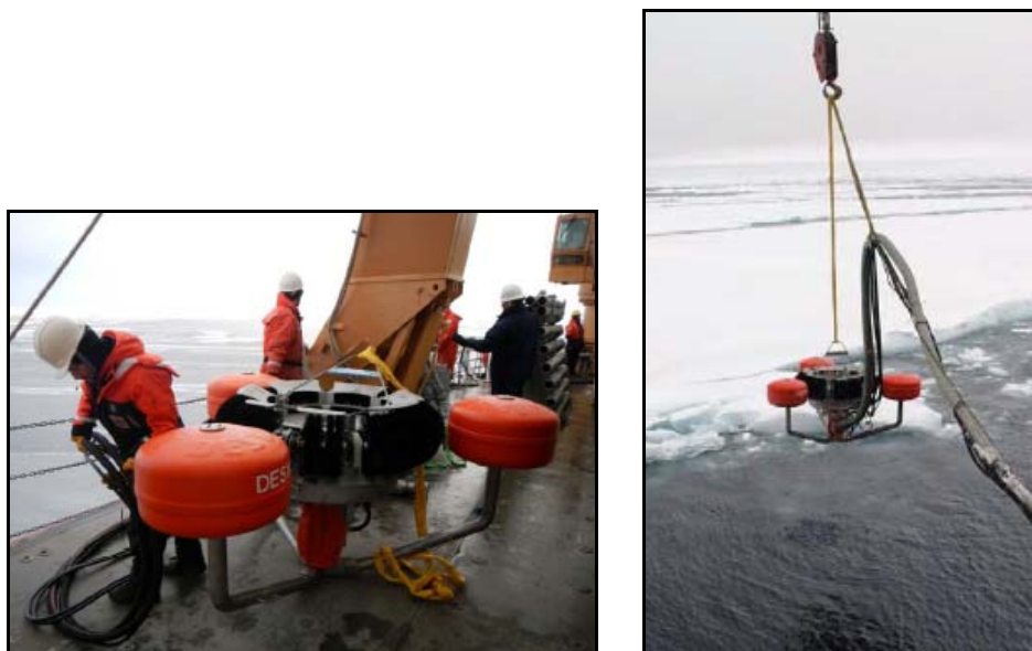
Figure A-2. Full configuration of DOP-Dual brush skimmer with stainless steel chemical hose (note that right photograph shows DOP-Dual with 3-inch hose).
