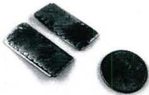
Figure 7: 3D printed IPMC samples: (left) thin membrane-shaped actuators and (middle and right) linear-type actuator consisting of layers of printed precursor material.
