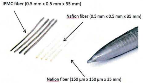
Figure 2: IPMC cilia-like fibers used in the image-based characterization experiments.
