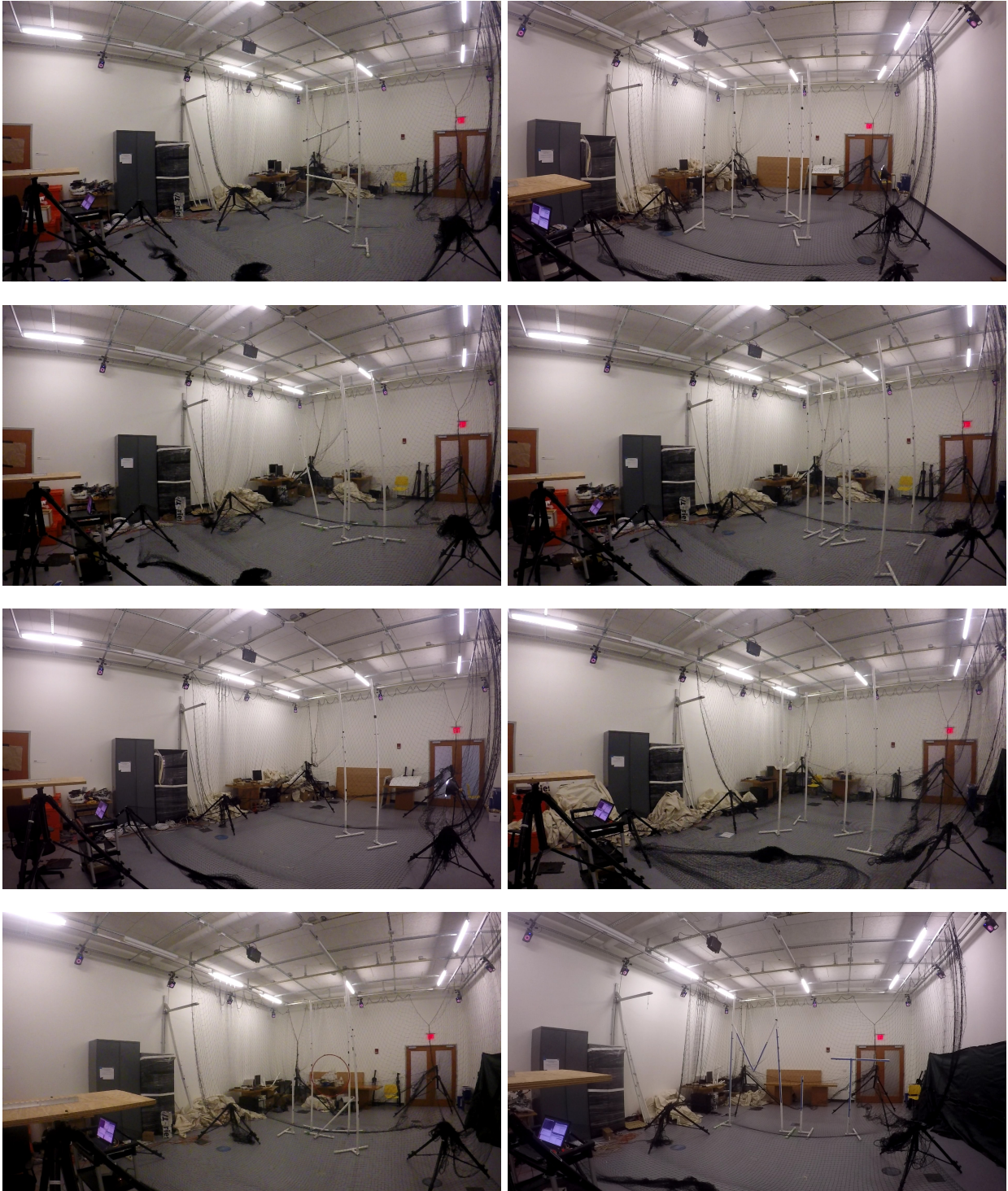
Figure 20: Environments 1-8 on which the online planning algorithm was tested. The obstacles include poles of different lengths in varying orientations and also a hoop of diameter equal to 0.9 m.
