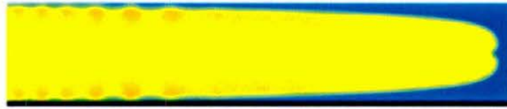
Figure 5. A laminar flame propagates down a smooth channel. Initially, before the hot spot is formed, and as the flow velocity increases (due to expansion and boundary-layer interactions), instabilities develop on the flame surface. This affects both the material inside the flame and the boundary layer.
