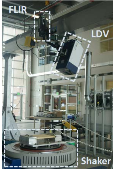
Figure 4. Labeled schematic of the experimental setup used under ambient environmental conditions
